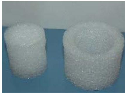
The inner core was inserted into the shell and the volume of the whole sample,  $V_{p1}$ , was obtained as **14.04 cm<sup>3</sup>** ( $\pm 0.17$ ). Since the top and bottom of the foam sheet is finished with the cells closed, those surfaces are not taken into account for correction calculations. In this particular case and due to the same cutouts height, the equation 6 can be presented in the form,
