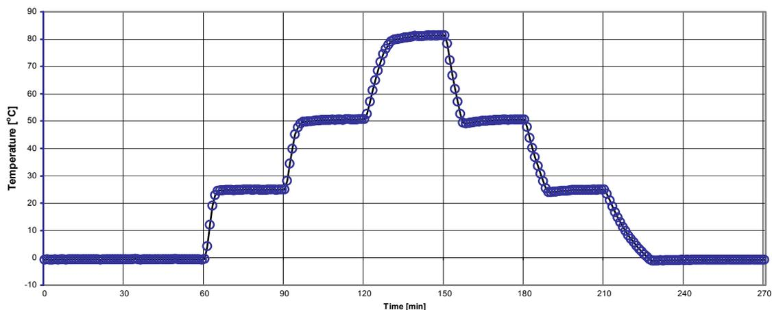
This figure shows equilibration dynamics for several large temperature steps in the increasing and decreasing direction versus time. The room temperature was varied often throughout the experiment by about 2 °C.
