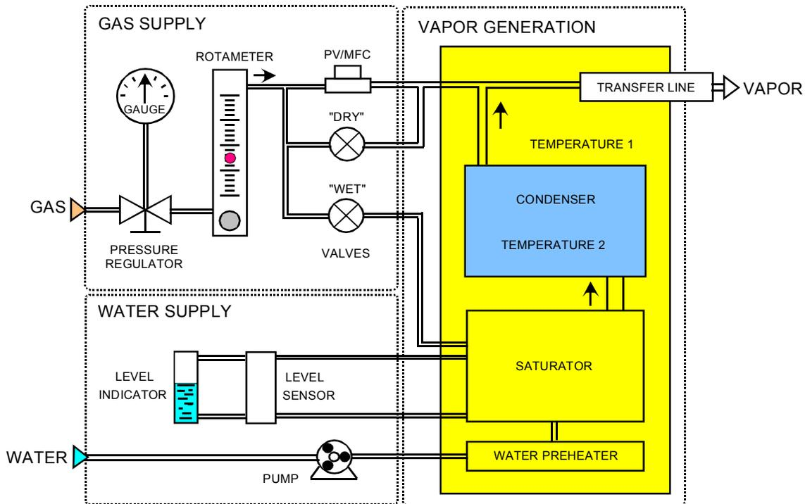
amount of flow bypassing the saturator increases. Thus, while maintaining the total flow constant, different ratios of dry gas flow to the saturated with water vapor gas flow can be obtained. An external RH sensor at the target needs to be used to monitor the output stream when the divided-flow method is employed.
