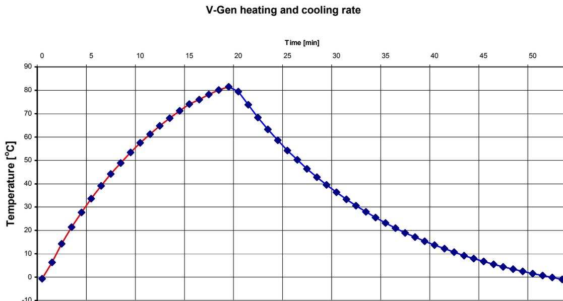
The figure shows the heating and cooling rate of the condenser chamber. The whole cycle of heating the chamber and cooling it back takes less than an hour for the 80°C temperature span.
