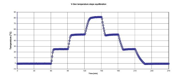
This figure shows equilibration dynamics for several large temperature steps in the increasing and decreasing direction versus time. The room temperature was varied often throughout the experiment by about  $2\,^{\circ}\text{C}$ .
