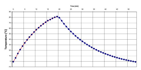
The figure shows the heating and cooling rate of the condenser chamber. The whole cycle of heating the chamber and cooling it back takes less than an hour for the  $80^{\circ}$ C temperature span.
