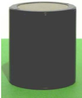
Large Sample Holder, Anodized, Fixed Porosity of 2, 5, 10, 20, or 40 microns:
