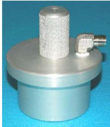
After inserting the volume reducing adapter in the sample chamber and securing it with the locking arm with screw, the packed bed cell can be connected to the pycnometer via a tubular link. The photo below shows a particular setup for measurement of flow rates, where the selected gas is supplied to the top of the cell using the precision pressure regulator of the pycnometer to set appropriate pressure values and measure the resulting flow amount from the bottom of the cell.
