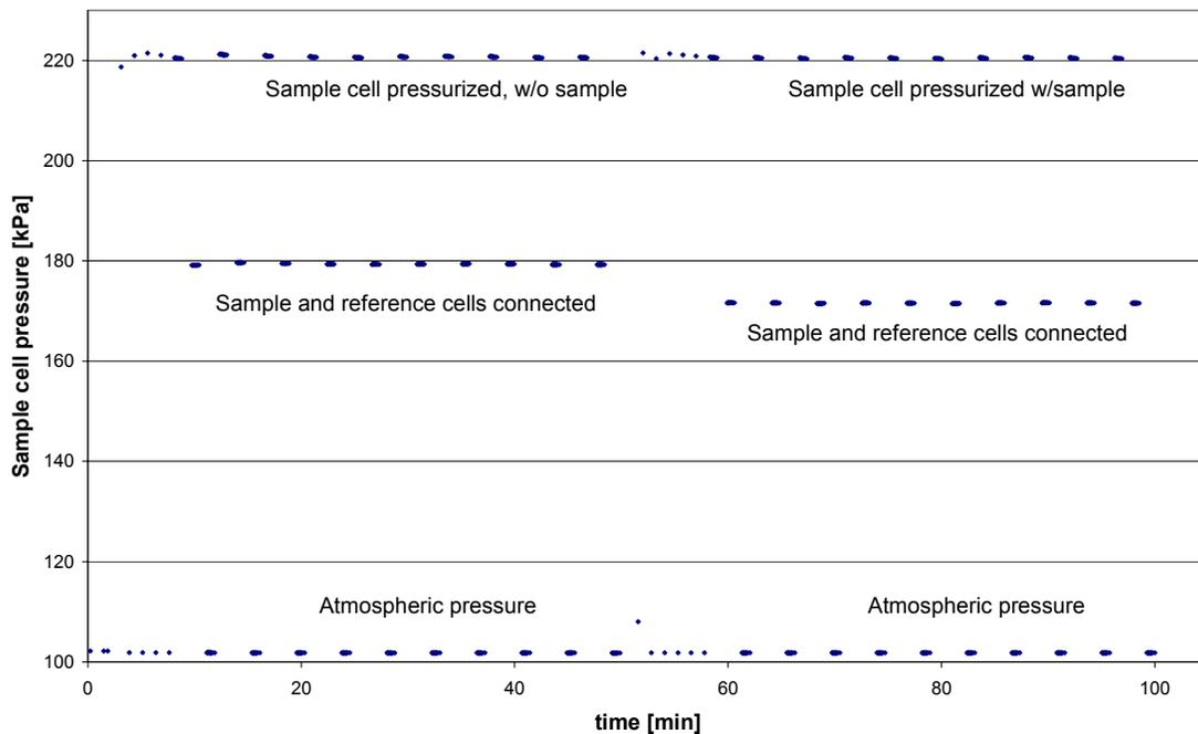
The above graph shows a typical isothermal run after the pycnometer has been calibrated. Initially, after placing the empty sample holder and closing the sample chamber, some preparatory steps like five pressure cycles (pressurization to some high value and depressurization to atmospheric pressure) take place to remove air/moisture from the sample chamber. Next, the actual process of measurement begins and in this
