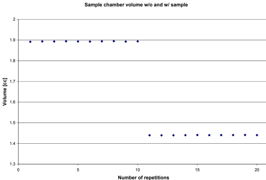
The above graph presents the calculated sample chamber volume after each measurement cycle. The difference between the two sets of repetitions is the sample volume. Knowing the sample mass, the true density is easily calculated and presented in the report for such experiment.
